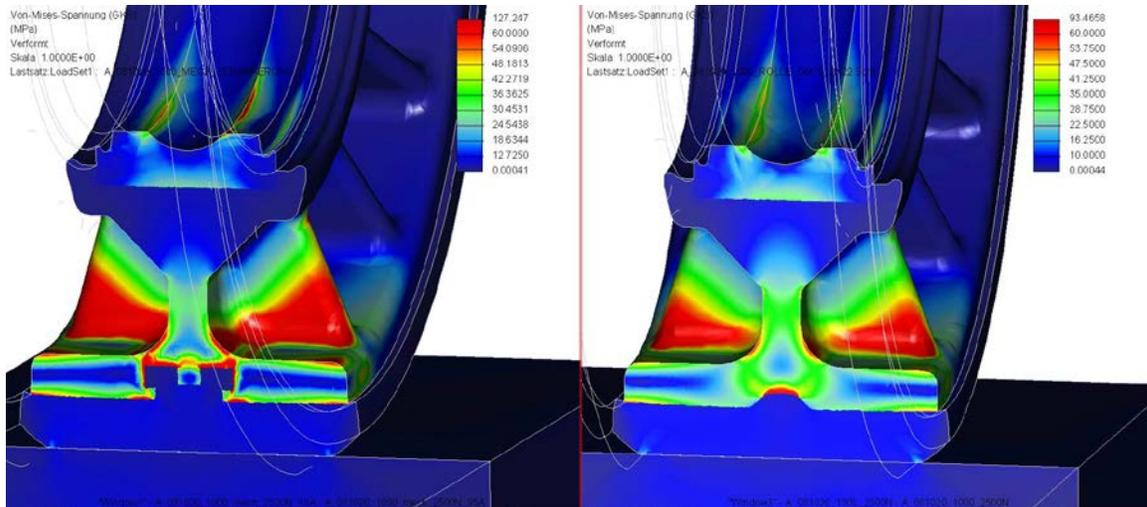
**Figure 1. Finite Elements Analysis of a roller with flanged design (left) and fused design (right)**
