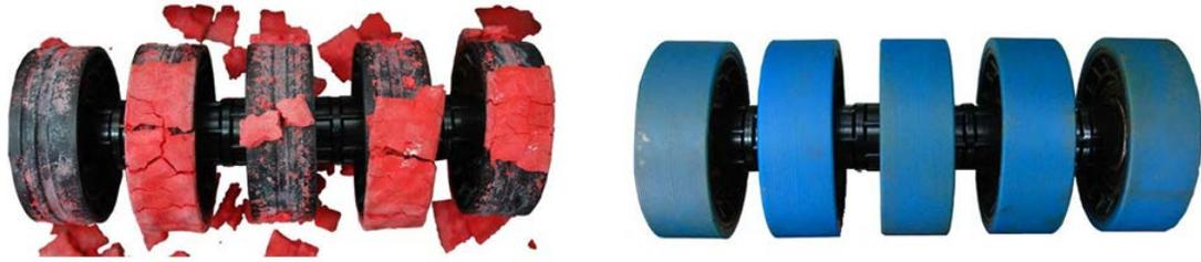
**Figure 3: Left side roller tire made of hydrolysis stabilized Polyester Urethane; Right side *Faigle* roller tire made of hydrolysis resistant Polyether Urethane**
