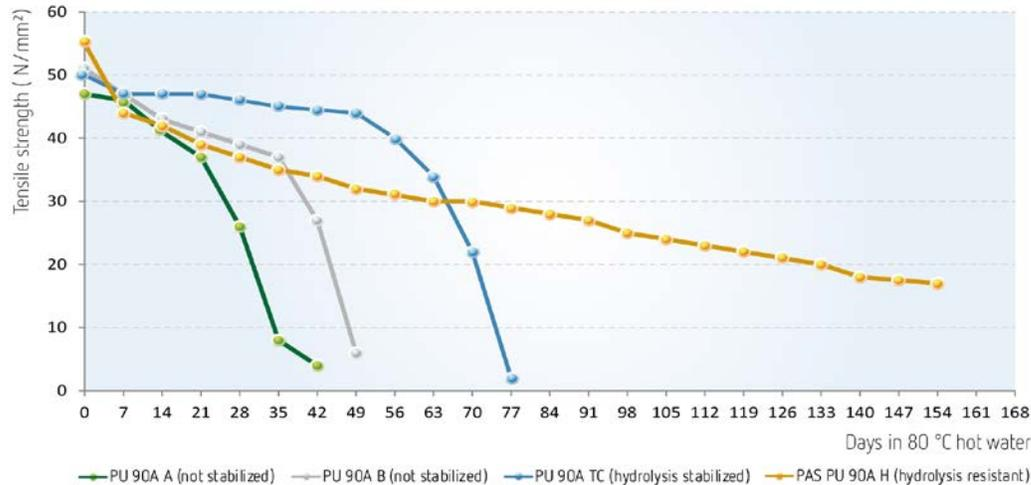
**Figure 4: Tensile strength of different TPU over days in 80°C hot water environment**
